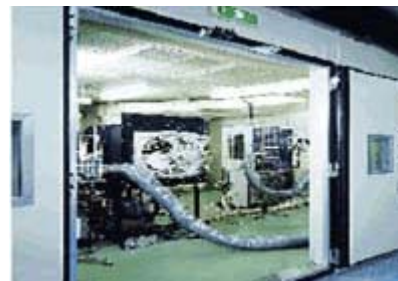
Thermal efficiency test for GHP
