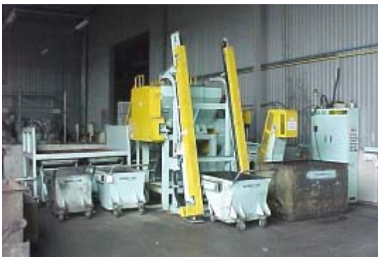
Compression and recycling equipment for polishing powder
