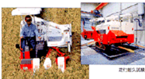
▲ Steering Wheel Operation Combine
